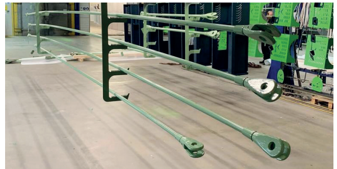
Tension rod systems of sizes M24-42, recently powder coated in RAL6021.
