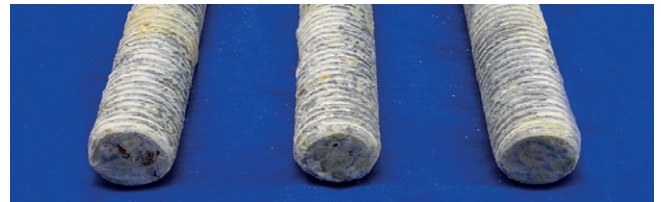
HMR bar threads after 480 hours of salt spray test.
