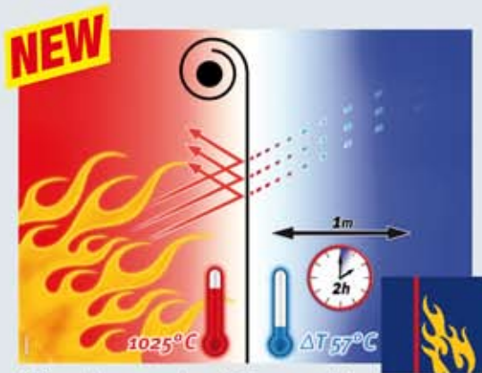
After 2 hours only 57°C in 1 m distance (schematic diagram EW120)
